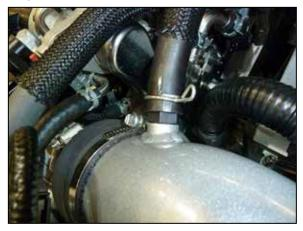
19. Connect the PCV hose to the fitting installed into the K&N $^{\odot}$  intake tube and secure with the factory spring clamp.
