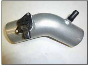
16. Remove the mass air sensor from the factory housing and install it into the  $K\&N^{\textcircled{o}}$  intake tube and secure with the provided hardware. Install the vent fitting into the  $K\&N^{\textcircled{o}}$  intake tube as shown. **NOTE: NPT fitting has tapered threads and only designed to be installed until hand tight, then tighten one rotation or when the fitting becomes difficult to return.**
