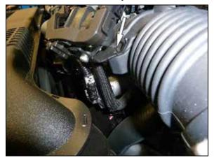
4. Unhook the solenoid bracket from the intake tube.
