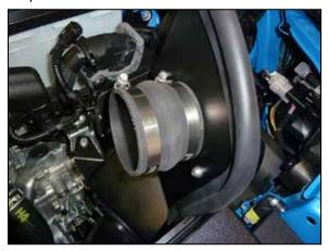
15. Install the provided hump coupler (087121) onto the filter adapter and secure with the provided hose clamp.
