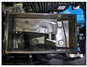
6. Remove the two bolts that secure the lower air filter housing and then remove the lower housing from the vehicle.
