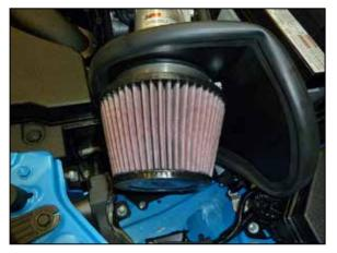
22. Install the K&N $^{\ensuremath{\$}}$  air filter and secure with the hose clamp.
