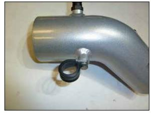
17. Install the provided cushion clamp onto the  $K\&N^{\circ}$  intake tube using the provided hardware.
