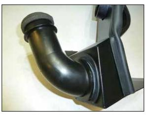
12. Install the 9-1/2" edge trim into the fresh air intake hole of the heat shield and then install the factory fresh air duct into the heat shield as shown.
